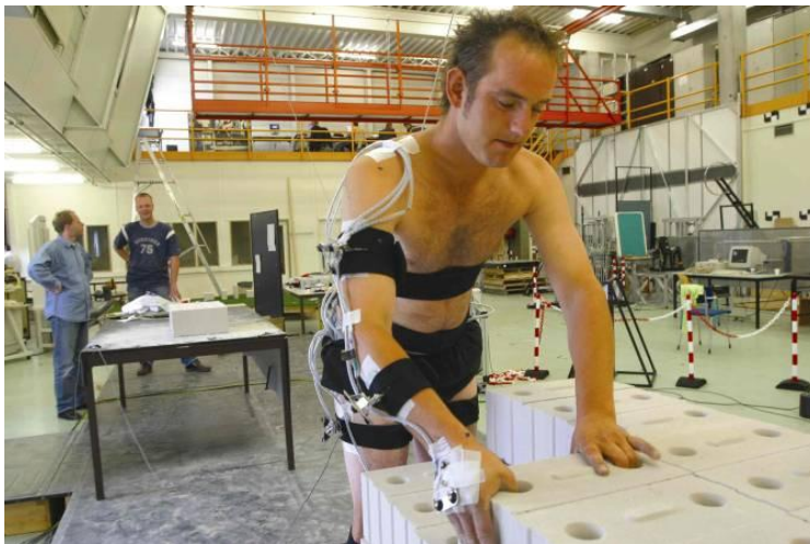
Figure 3. A laboratory study measuring the biomechanical load on the low back based on data about the weight of the object and the body posture and movements.
